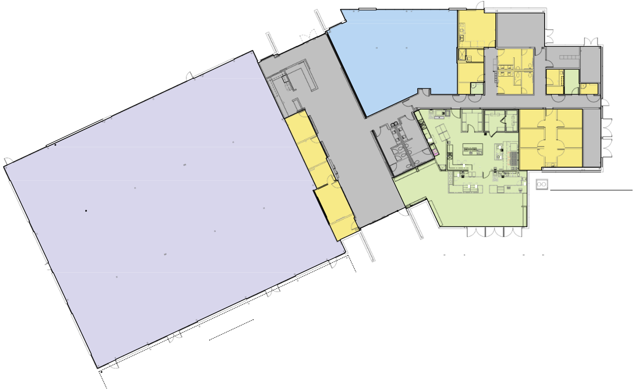
Figure 3: Area 1 Outpatient, Support Services & Kitchen/Café Building. Kitchen & Café space shown in green at 2,520 SF (Kitchen: 1,255 SF, Serving: 311 SF, Café Seating: 954 SF)
